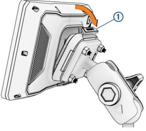
Push the top of the device forward until it snaps into place.The latch ① on the mount stays up after you insert the device.
