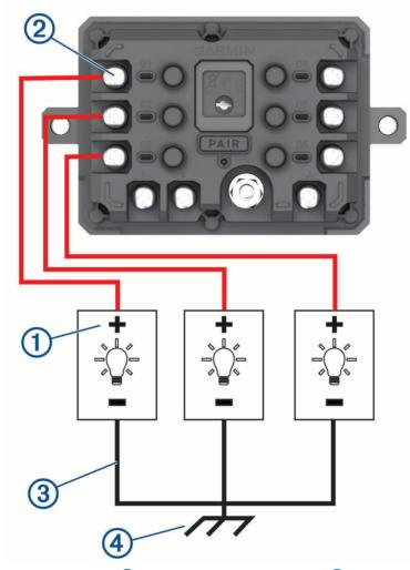
2 Connect the negative or ground wire ③ to an unpainted ground stud ④ on the vehicle frame, to a ground distribution block, or directly to the negative terminal on the battery.
