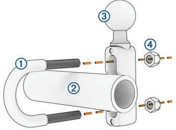
2 Tighten the nuts 4 to secure the base.
