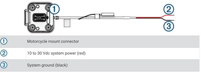
**NOTE:** Additional parts are included with the device to provide more installation and wiring options. Contact an experienced installer for more information about using these parts with your motorcycle.
